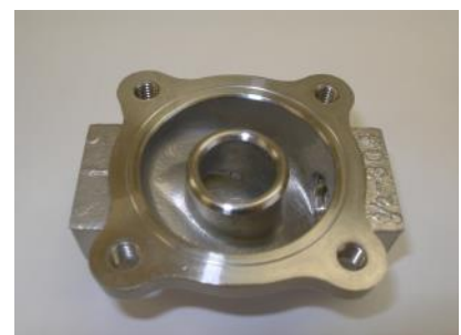
Figure 7: Lower body. Debris in the lip of the inner chamber may cause valve malfunction
