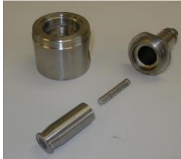
Figure 2: Direct acting valve with all components shown. Debris on the plunger may lead to valve malfunction.
